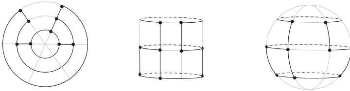
Figure 1: An ortho-radial drawing of a graph and its corresponding drawings on a cylinder and a sphere.
